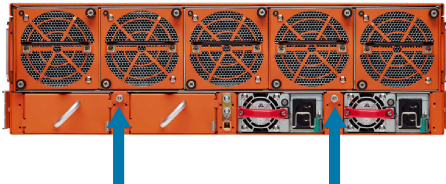
Figure 4-10: Fan Tray Screw Location on GigaVUE-HC3 Rear
