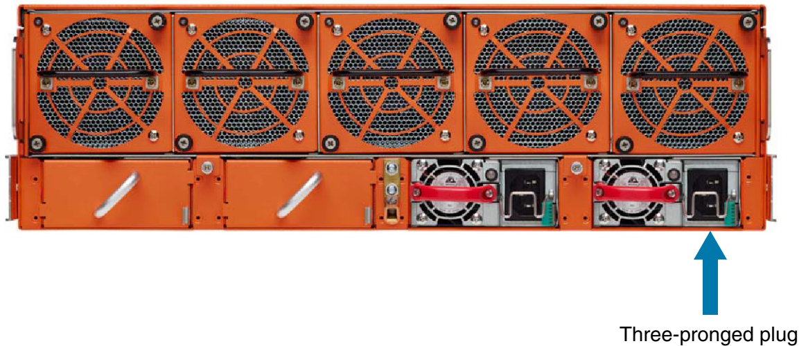
Figure 4-2: Connecting AC Power
